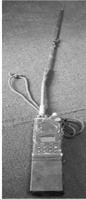
Tadiran RT-7106 (PRC-710) tactical VHF/FM radio transceiver. The attached TEL-718B battery unit is visible at the base.
