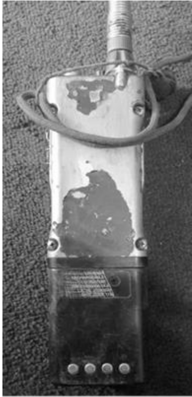
Tadiran RT-7106 (PRC-710) tactical VHF/FM radio transceiver. The attached TEL-718B battery unit is visible at the base.
